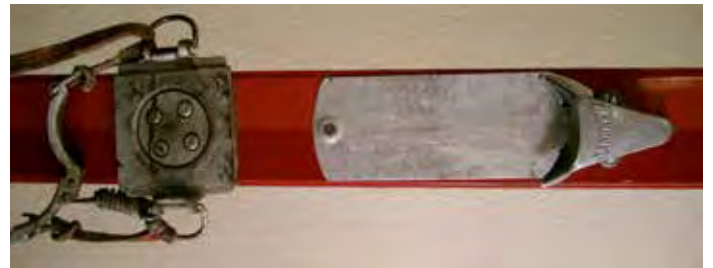
The Marker Simplex toe piece and turntable with longthong
